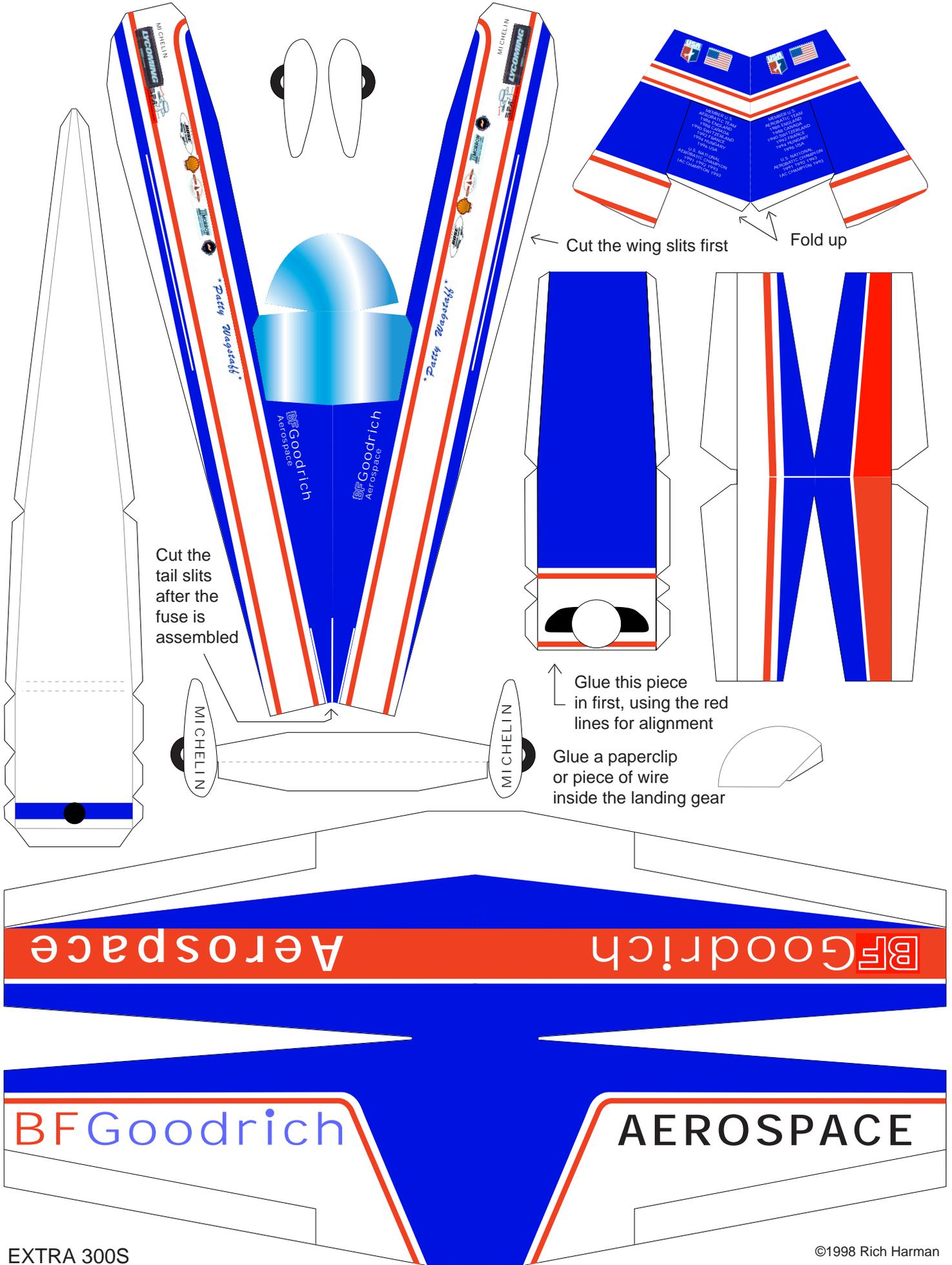
Cut the tail slits after the fuse is assembled
